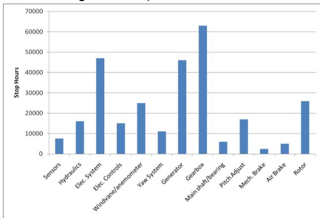
*Fig. 1 Downtime hours accumulated from 2003 to 2007 for wind turbines operating in Germany[1]*
