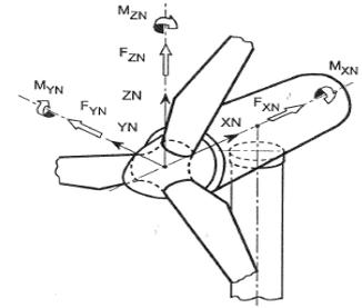
Fig. 3 Loads & Working System of Axis[3]
