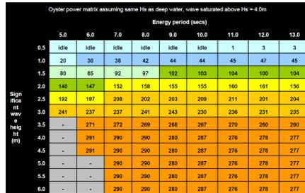
Figure 4 – Oyster device power matrix
