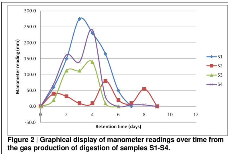
**Figure 2 | Graphical display of manometer readings over time from the gas production of digestion of samples S1-S4.**
