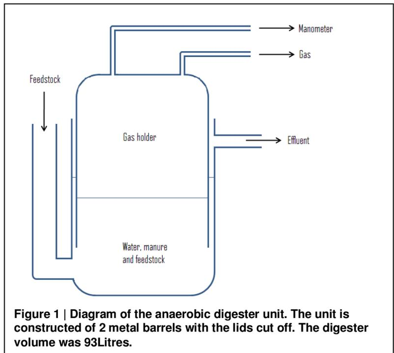
Figure 1 | Diagram of the anaerobic digester unit. The unit is constructed of 2 metal barrels with the lids cut off. The digester volume was 93Litres.
