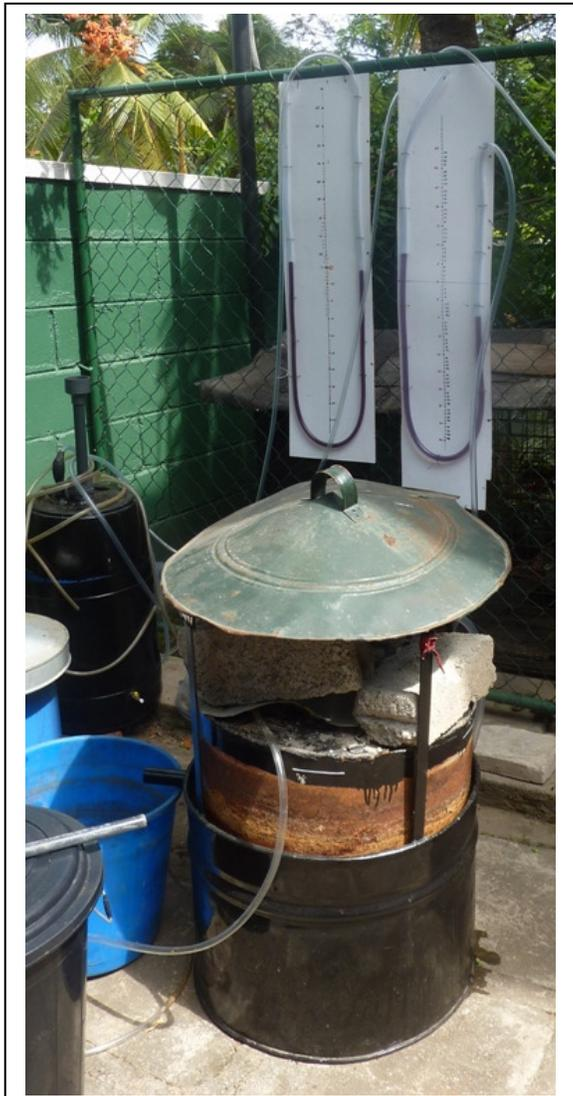
Image 1 | Photograph of the trial digester unit and the manometer
