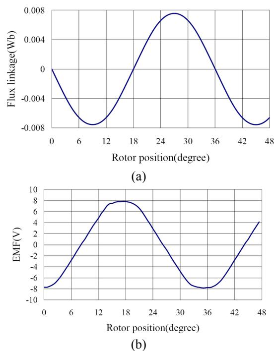
Fig.2: (a) Phase flux linkage waveform, (b) Phase back EMF waveform
