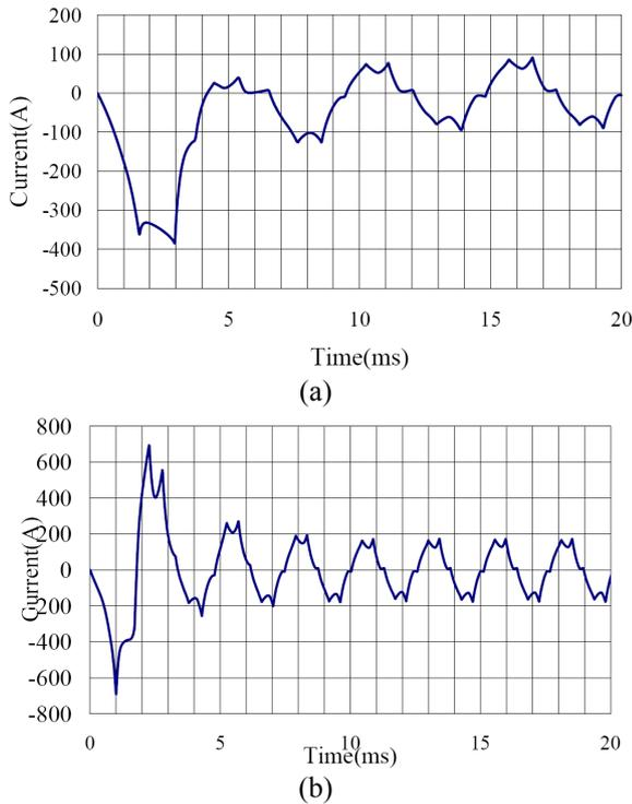
Fig. 6 (a) Starting current with windings in series, (b) Starting current with windings in parallel
