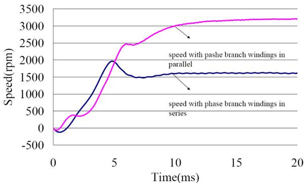
Fig. 7. Extended speeds under rated torque operation
