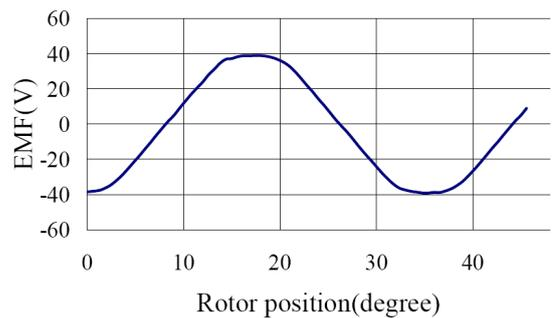
Fig.9. Back-EMF waveform at 5000 rpm
