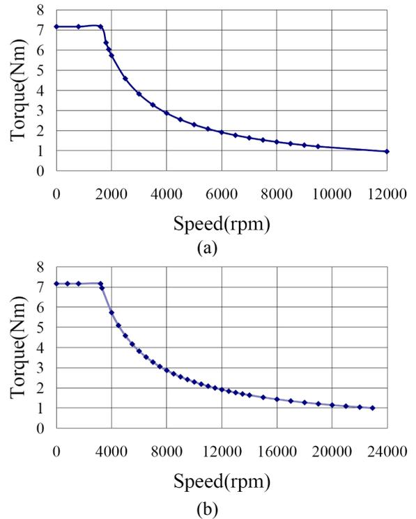
Fig. 8(a) Extended speed under constant power operation with windings in series, (b) Extended speed under constant power operation with windings in parallel
