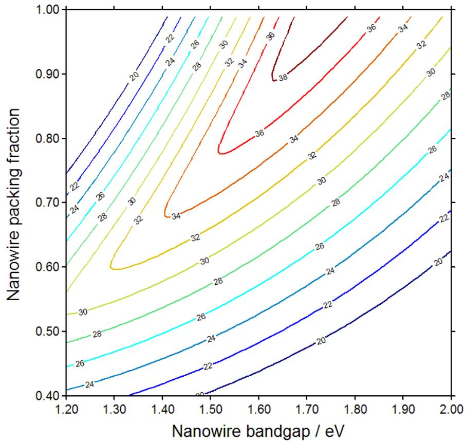
Relative improvement in efficiency over silicon cell for GaAs nanowires with ideal single AR coat
