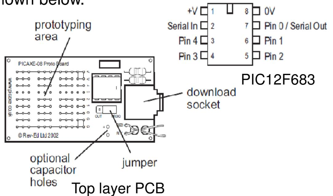
The PICAXE-08 proto board provides a rapid development system for the 8pin microcontroller system. It provides the basic download circuit beside a small proto typing area for connection of input / output circuits to the PICAXE-08 pins as shown above.
