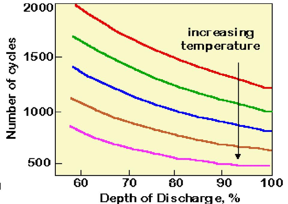
The capacity of a lead acid battery is reduced at low temperature operation; high temperature operation increases the aging rate of the battery. The impact on battery charging relates to the temperature of the battery.
