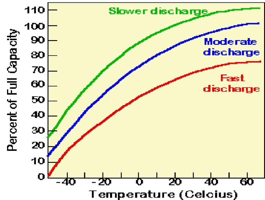
Relationship between battery capacity, temperature and lifetime for a deep-cycle battery.
