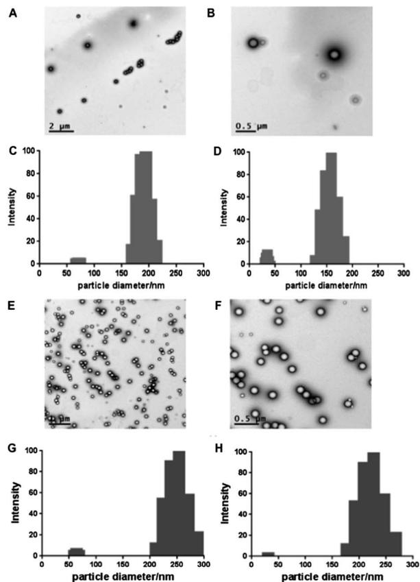
Fig. 3 (A and B) TEM micrographs (stained with uranyl formate) of HB-PAMPS PBMA latex particles. (C) HB-A particle size distribution and (D) HB-B particle size distribution. (E and F) TEM micrographs (stained with uranyl formate) of L-PAMPS PBMA latex particles. (G) L-A particle size distribution and (H) L-B particle size distribution.
