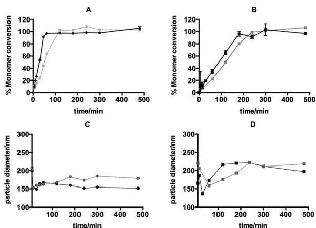
Fig. 4 Plots of conversion/time and particle size/time for emulsion polymerisations of BMA containing HB-PAMPS or L-PAMPS. (A) Conversion of BMA and C, average particle diameter *versus* time for polymerisations containing HB-PAMPS. (B) Conversion of BMA and D, average particle diameter *versus* time for polymerisations containing L-PAMPS: ● HB-PAMPS 1 g; ● HB-PAMPS 4 g; ■ L-PAMPS 1 g; ■ L-PAMPS 4 g.
