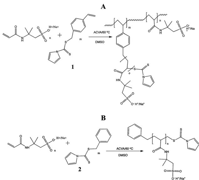
Fig. 1 Synthesis of (A) HB-PAMPS by RAFT-SCVP and (B) L-PAMPS by RAFT.
