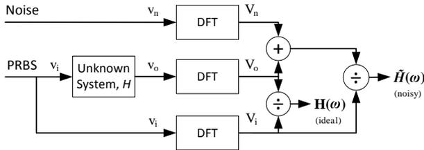
**Fig. 1** Process for system identification using PRBS showing noiseless output,  $H(\omega)$ , and noisy output,  $\tilde{H}(\omega)$ .
