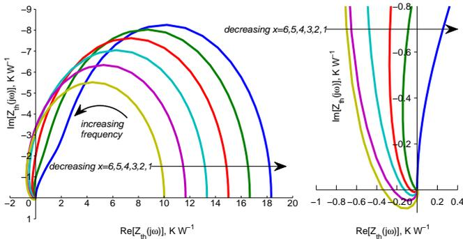
**Fig. 5** Nyquist plots of single material Cauer network approximation with transfer impedance taken at different nodes,  $x$
