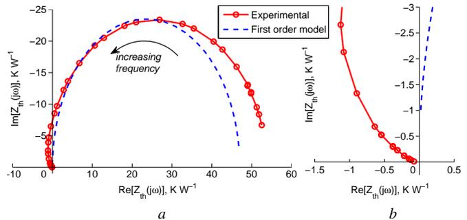
**Fig. 2** Nyquist plot of experimental transfer impedance spectrum for a TO220 device with fitted first order model
