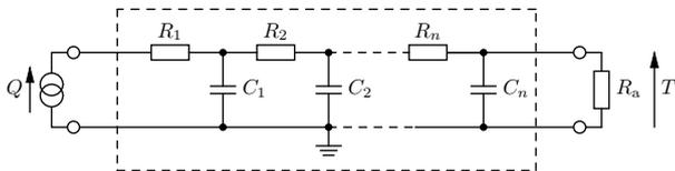
**Fig. 1** Two-port Cauer network with heat source,  $Q$ , and ambient connection,  $R_a$
