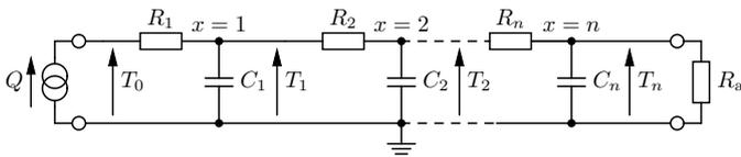
**Fig. 4** Cauer two-port network with temperature measurements taken at various points along the material.
