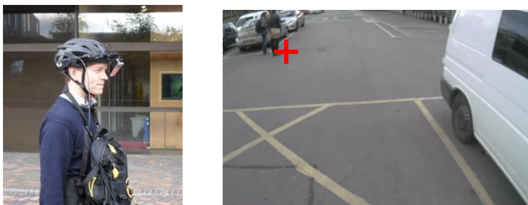
Figure 1 – SMI iView X HED mobile eye tracking system (left) and screenshot from recorded video (right). The red cursor shows current gaze location (amplified for this image).
