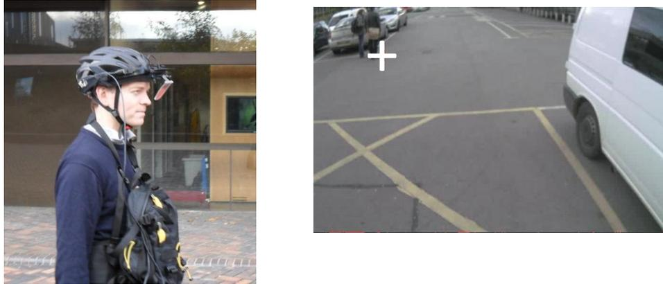
**Figure 1 – Eye-tracking apparatus and an example of the video record – the cross (amplified for this image) indicates the point of visual fixation**
