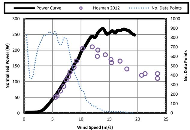
Figure 9: Relationship between the number of data points and the reliability of the measured data.
