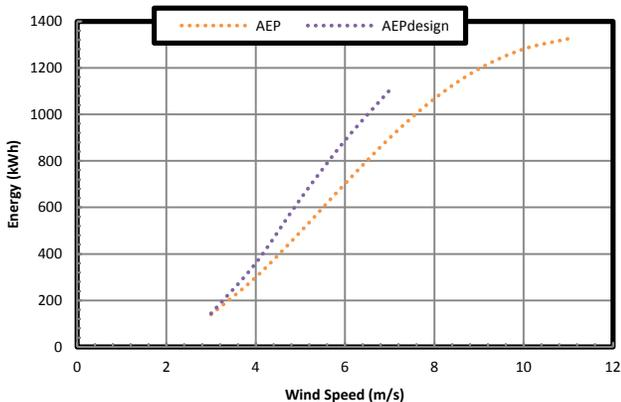
Figure 8: Comparison of the measured Annual Energy Production (AEP) with the design values, as stated in *A Wind Turbine Recipe Book* [1]
