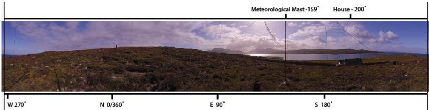
Figure 6: 360° panoramic photograph of test site relating locations of potentially significant obstacles to flow onto the wind turbine.
