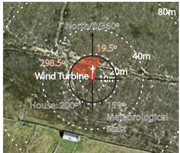
Figure 5: Satellite photograph of the site showing radial contours of distance from wind turbine (white) and the excluded sector when the meteorological mast is downstream of the wind turbine (red). Image courtesy of Google Maps.
