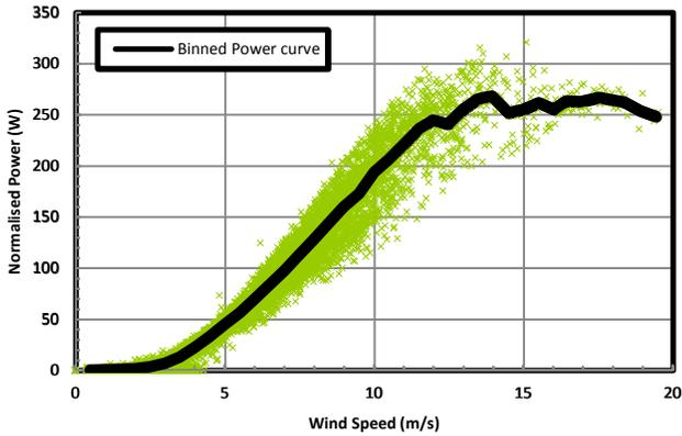
Figure 7: Scatter plot of all data (after removing samples taken when anemometer in wake of turbine) with binned power curve.
