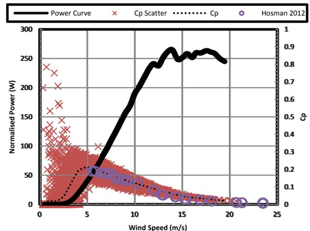
Figure 10: Scatter plot of power coefficient,  $C_p$ , using all data (after removing samples taken when anemometer in wake of turbine) with binned power curve.
