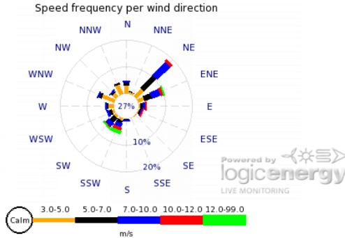
**Figure 1:** Wind rose for the Glasshouse test site during the measurement period. Image courtesy of Logic Energy.
