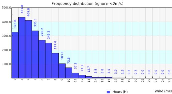
**Figure 2:** Wind speed frequency distribution for the Glasshouse test site during the measurement period. Image courtesy of Logic Energy.
