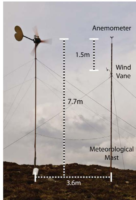
**Figure 3:** Photograph of the meteorological mast showing its proximity to the wind turbine.
