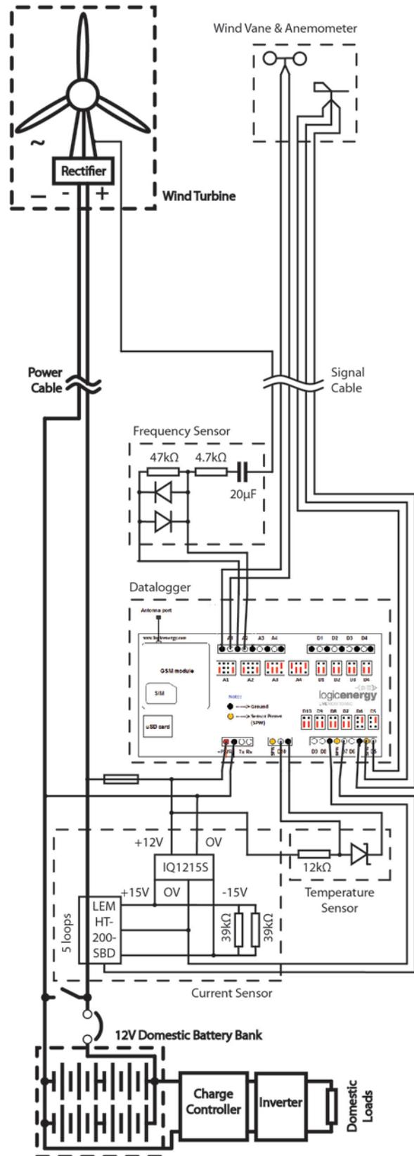
**Figure 4:** Wiring diagram of the data logging equipment installed on the Glasshouse wind turbine. LeNET image courtesy of Logic Energy [3].
