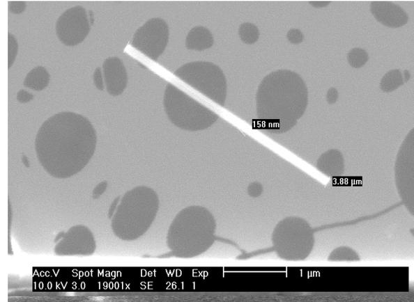
FIG. 4: The wire studied in detail with TEM, with approximate diameter 160nm and length  $3.9\mu\text{m}$ .
