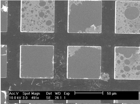
FIG. 3: SEM image of a TEM grid after an initial attempt to transfer the NWs onto the TEM grid using the ‘brute force’ method. The circular holes visible in the film are a natural part of the film, however the central squares of the grid have little or no film since it has been torn away during the process of knocking over the NWs. A high density of nanowires is visible on the copper grid near the squares where the film has been torn away.
