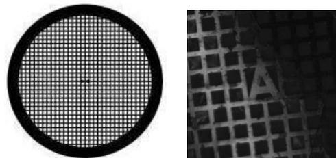
FIG. 1: The TEM grids used in the investigation. The grid is roughly 3mm in diameter and the centre is marked with an 'A' as shown which assists locating the wires.
