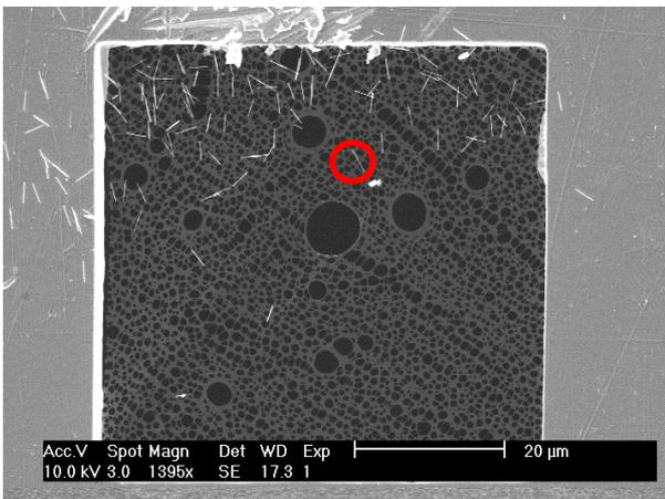
FIG 10: The wires selected for TEM investigation. The red circle shows the wire selected for more detailed study, which is approximately  $3.3\mu\text{m}$  in length with a diameter of 105nm.
