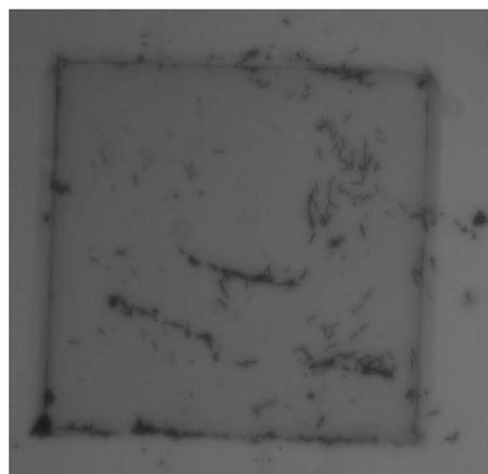
FIG 2. Optical image of the array after wires were knocked over within a droplet. It can be seen that some wires are knocked over without being moved greatly, but that there is also a large amount of aggregation of wires.
