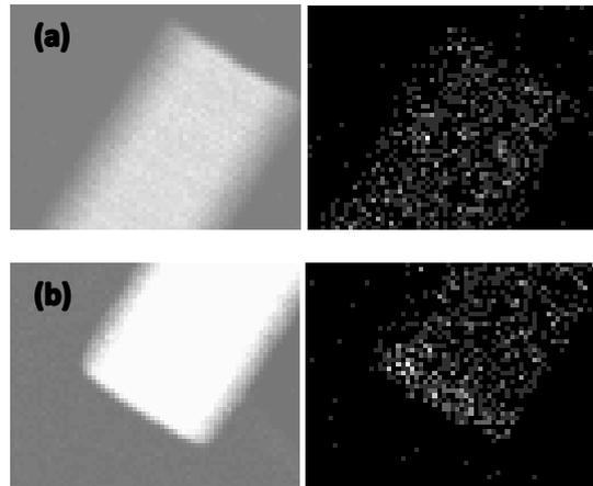
FIG 13: Images of the two ends of the wire under investigation. The images with a grey background show the wire, whilst the images with a black background show only the signal detected from phosphorous. Images (a) correspond to the end of the wire where it broke off from the substrate. Images (b) correspond to the 'top' end of the wire where a phosphorous cap was grown, as can be seen by the increase in phosphorous signal at the very end of the wire.
