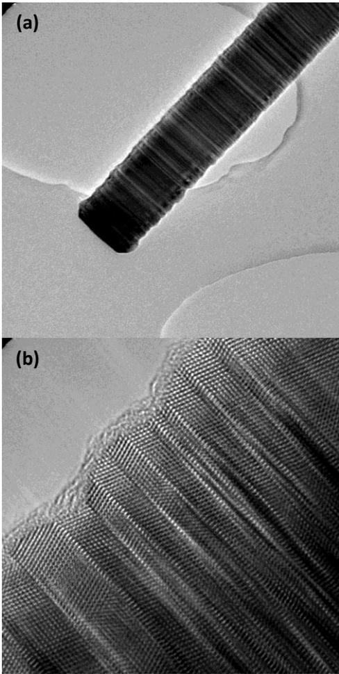
FIG 5: High resolution TEM Images showing stacking faults. (a) is 2000 times magnification, whilst (b) is 50000 times magnification.
