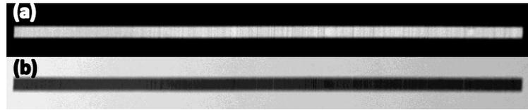
FIG 11: Dark field (a) and bright field (b) scanning TEM images of the nanowire under investigation. Again stacking faults are clearly visible.
