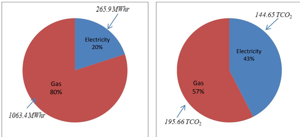
**Figure 18: Actual Energy Consumption & Emissions for Crookesmoor**
