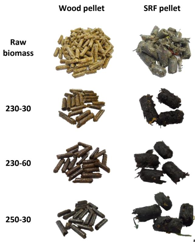
\*SRF-250-30 was only reacted for ~5 min after which time the reaction was abandoned. Photograph is of product after this reduced time.
