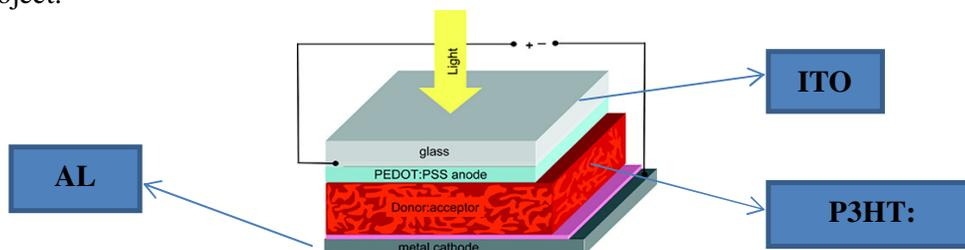
Figure 2: A typical BHJ organic solar cell [2]
