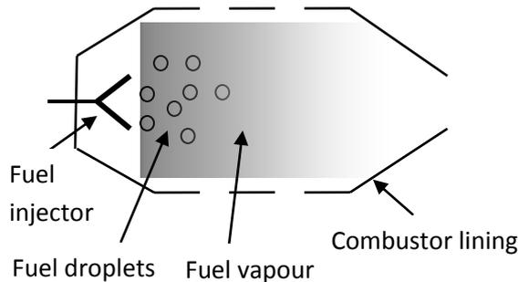
**Figure 1: Fuel evaporation within the combustor**
