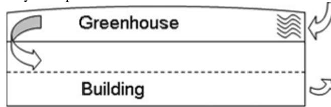
**Fig1. Evaporatively cooled hydroponic greenhouse on top of a hypothetical 2-story building, from [13].**
