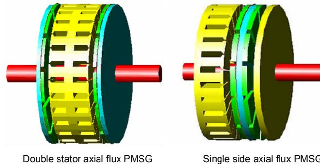
*Figure 3 Double stator and single side axial flux wind PMSG*
