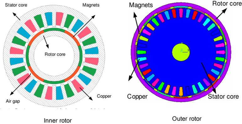
Figure 1 Inner and outer rotor radial-flux PM generators
