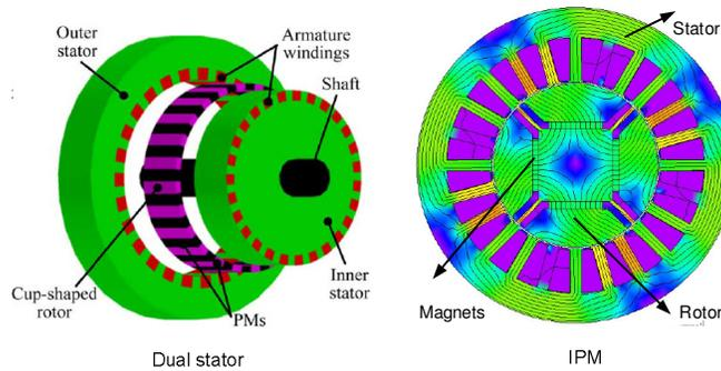
Figure 2 Dual stator and IPM radial-flux PM generators
