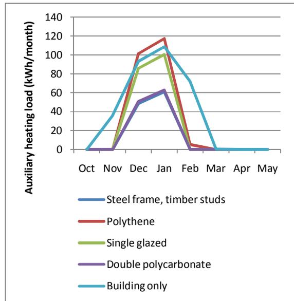
Figure 4. Auxiliary heating load of building with different greenhouse constructions.
