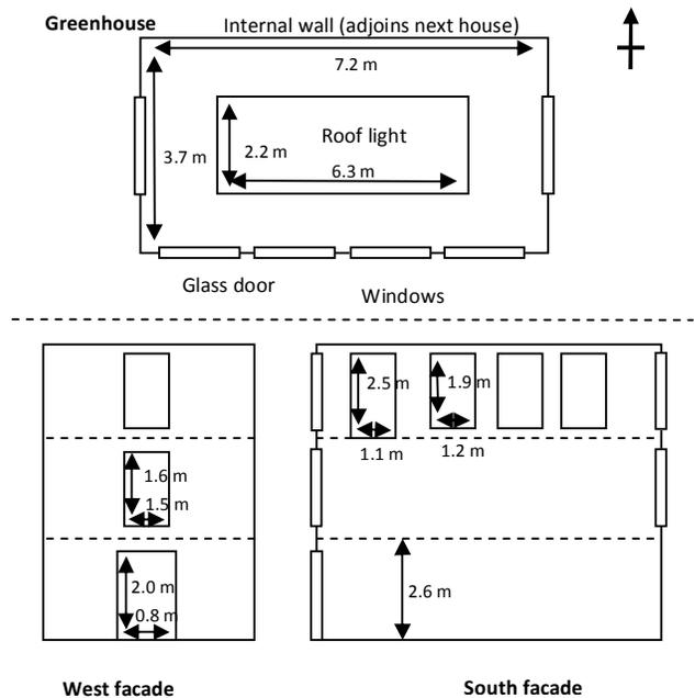
**Figure 1. Schematic diagram of greenhouse and office layout.**
