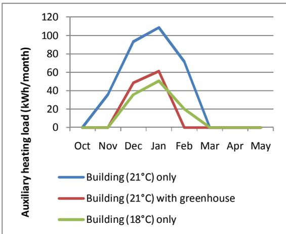
Figure 3. Auxiliary heating load of the building with and without a greenhouse.
